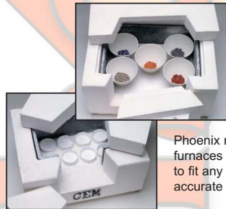
Phoenix microwave-powered muffle furnaces are available in configurations to fit any ashing need. They are fast, accurate and easy-to-use.
