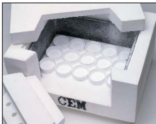
The High Capacity 1000 °C furnace holds up to 15 (25-mL) crucibles and is ideal for the laboratory needing greater throughput.
